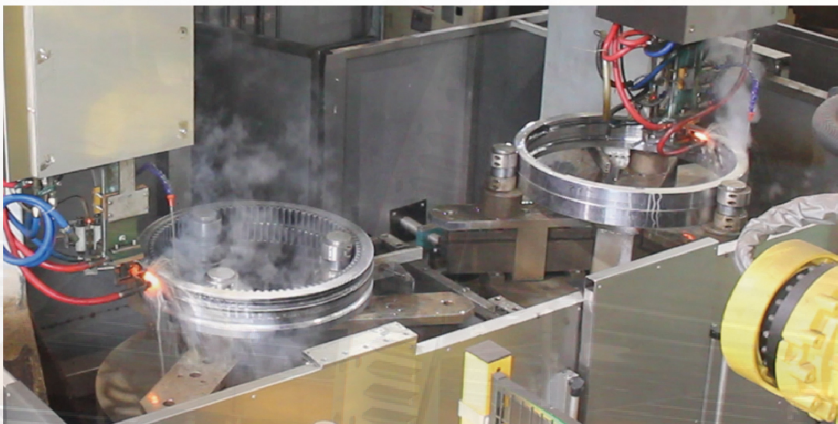
双工位双感应器双圈淬火，效率倍增 Dual-station, dual-inductor and dual workpieces hardening, double efficiency
