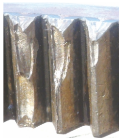
Figure 4 Title: Failure of gear with 37 degree chamfer
