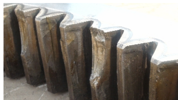
Figure 4 Title: Failure of gear with 37 degree chamfer
